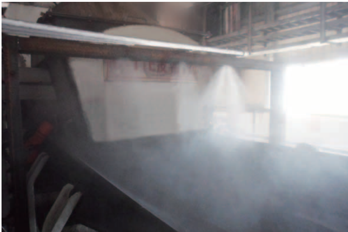
导料槽尾部抑尘 Tail Dust Suppression of Hopper Chute
