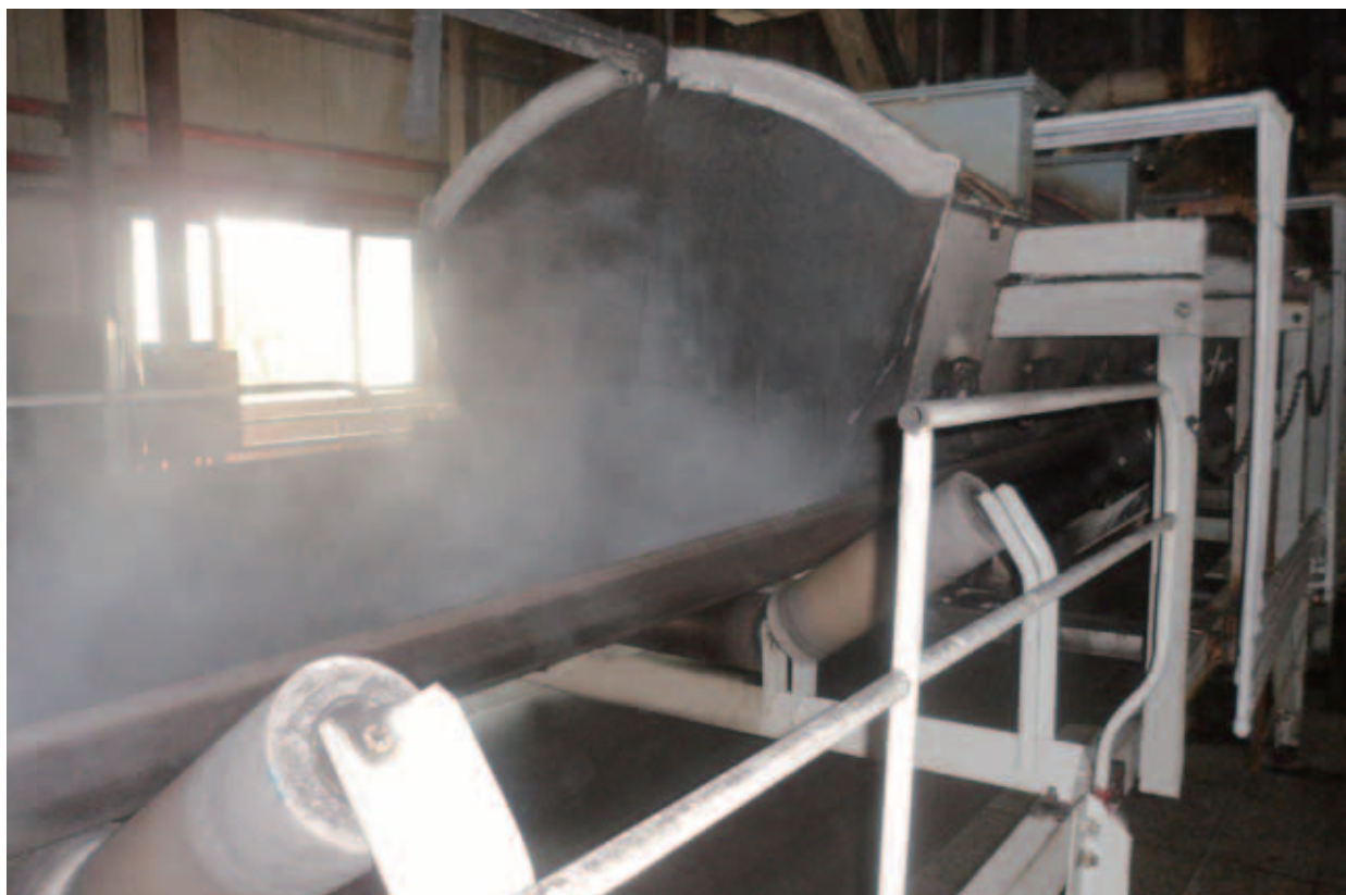
导料槽出口抑尘 Dust Suppression Exit of hopper Chute
